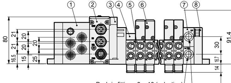
Push-in fitting  $\phi 8$ ,  $\phi 10$  (selection)
