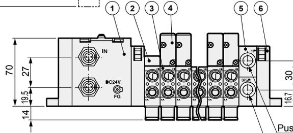
Push-in fitting  $\phi 4, \phi 6, \phi 8$  (selection)
