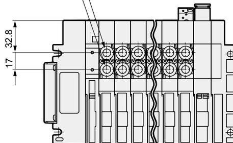
● Radial push-in fitting for supply and exhaust block (upward)
