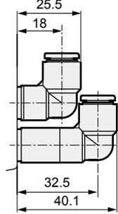
● Radial push-in fitting for supply and exhaust block (upward)
