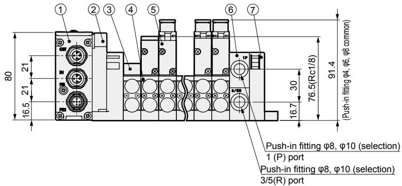
● Radial push-in fitting for supply and exhaust block (upward)
