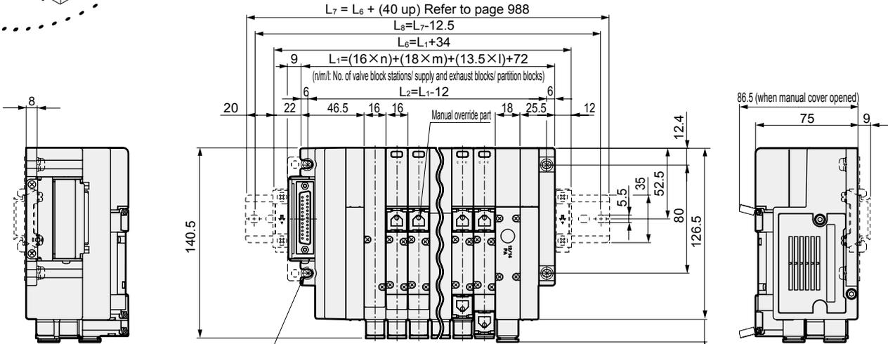
4-M5 mounting hole (for direct mounting)
