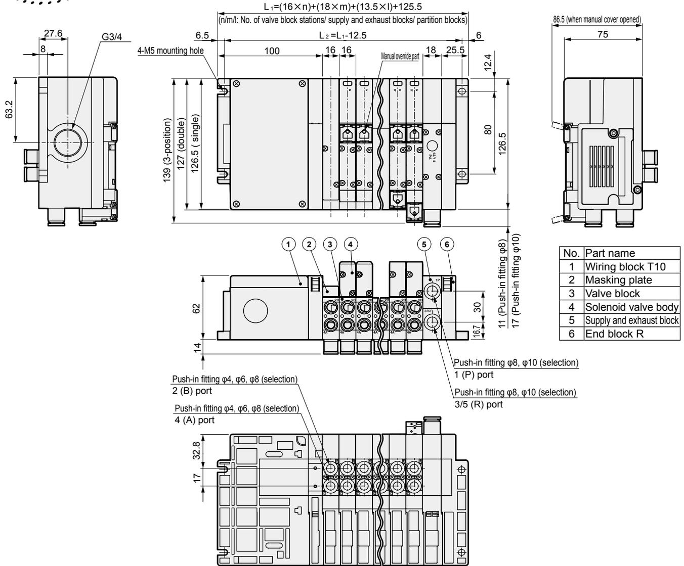
● Radial push-in fitting for supply and exhaust block (upward)
